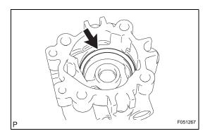
(c) Remove the O-ring from the vane pump housing front.
