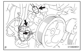
(c) Remove the 2 bolts and the vane pump assembly.
