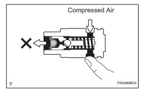
(b) Check the flow control valve for leakage. Close one of the holes and apply compressed air of 392 to 490 kPa (4 to 5 kgf/cm², 57 to 71 psi) to the hole on the opposite side. Confirm that the air does not flow out from the end holes.
